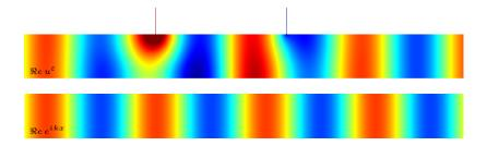
• Here the device is designed to obtain a phase shift approx. equal to  $\pi/4$ .
