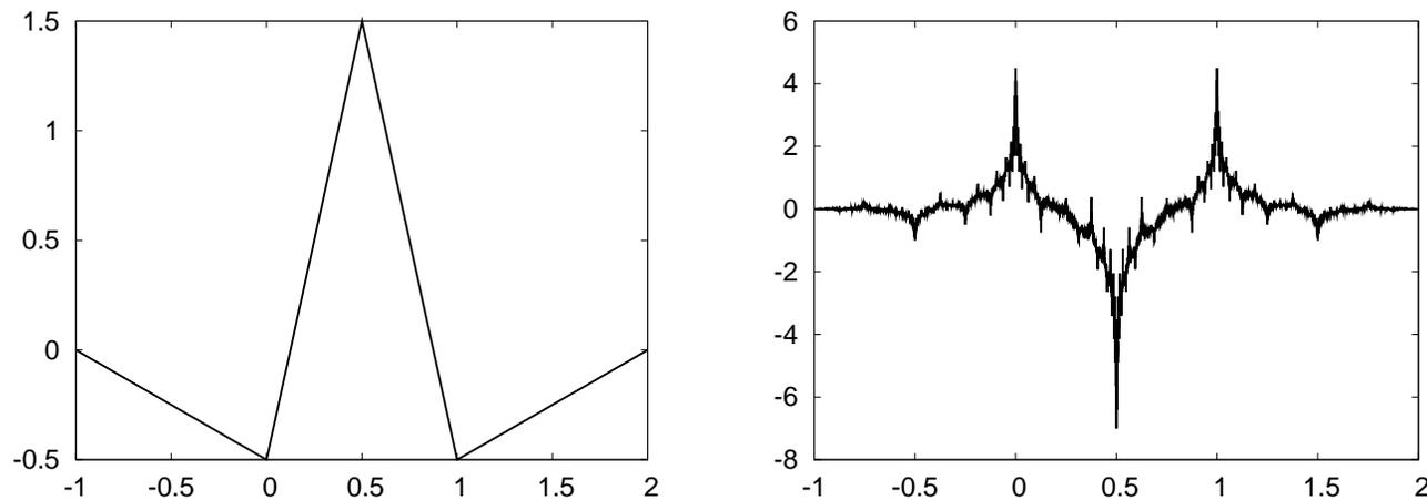
Figure 2: Corresponding primal and dual wavelet
